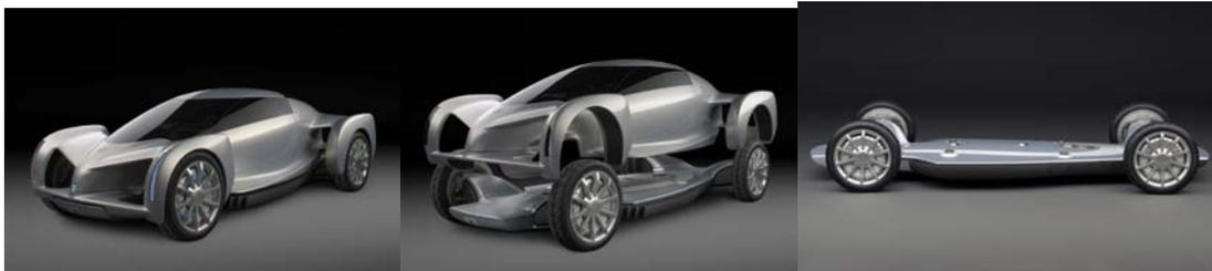
Fig. 2. The Autonomy “skateboard prototype
